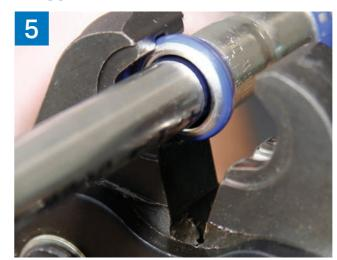
Must use correctly sized jaw/collar. Fittings must be aligned correctly in jaw/collar. Ensure insertion depth is met before pressing.
