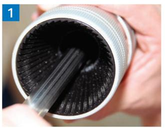
Cut the pipe to length and deburr inside and out so as not to damage the seal ring. Clean chips from the pipe end.
