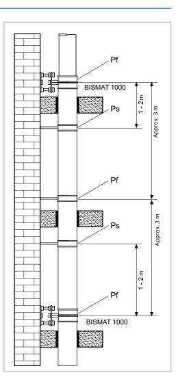
**Pf** - fixed point – Bismat 1000 clamping ring or standard clamping ring with a rubber insert
