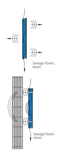
For the noise protection to be effective, the levels of the above types of noise should be reduced. With the application of the Ultra dB soundproof indoor sewage system, the subjective perceived level of noise is considerably reduced as compared to the noise coming from standard drain pipes. Thanks to the use of the double-layer pipe wall, the airborne noise is considerably attenuated and it becomes almost inaudible.
