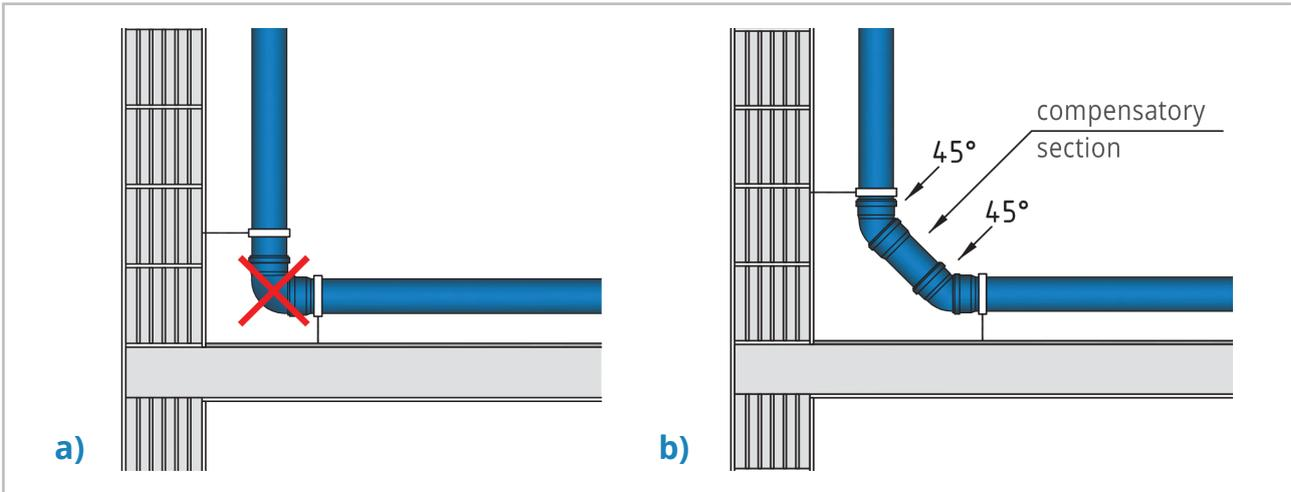
**Fig. 2. Transition of waste stack to horizontal branch drain**
