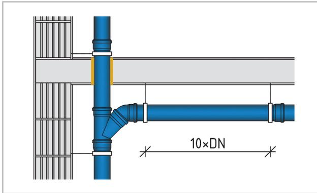
**Fig. 4** Distance between clamping rings on horizontal branch
