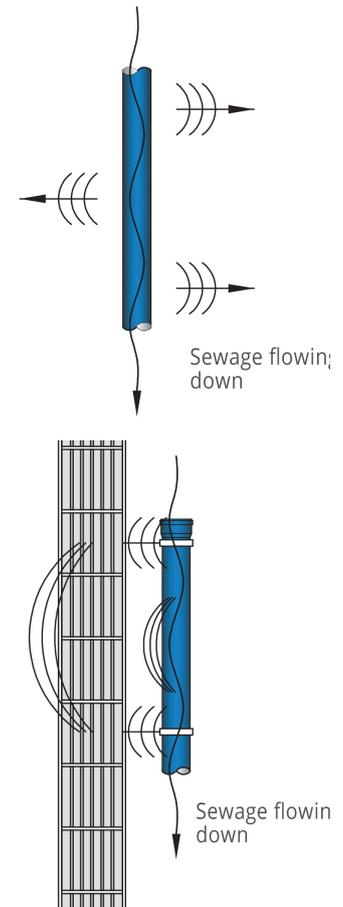
For the noise protection to be effective, the levels of the above types of noise should be reduced. With the application of the Ultra dB soundproof indoor sewage system, the subjective perceived level of noise is considerably reduced as compared to the noise coming from standard drain pipes. Thanks to the use of the double-layer pipe wall, the airborne noise is considerably attenuated and it becomes almost inaudible.
