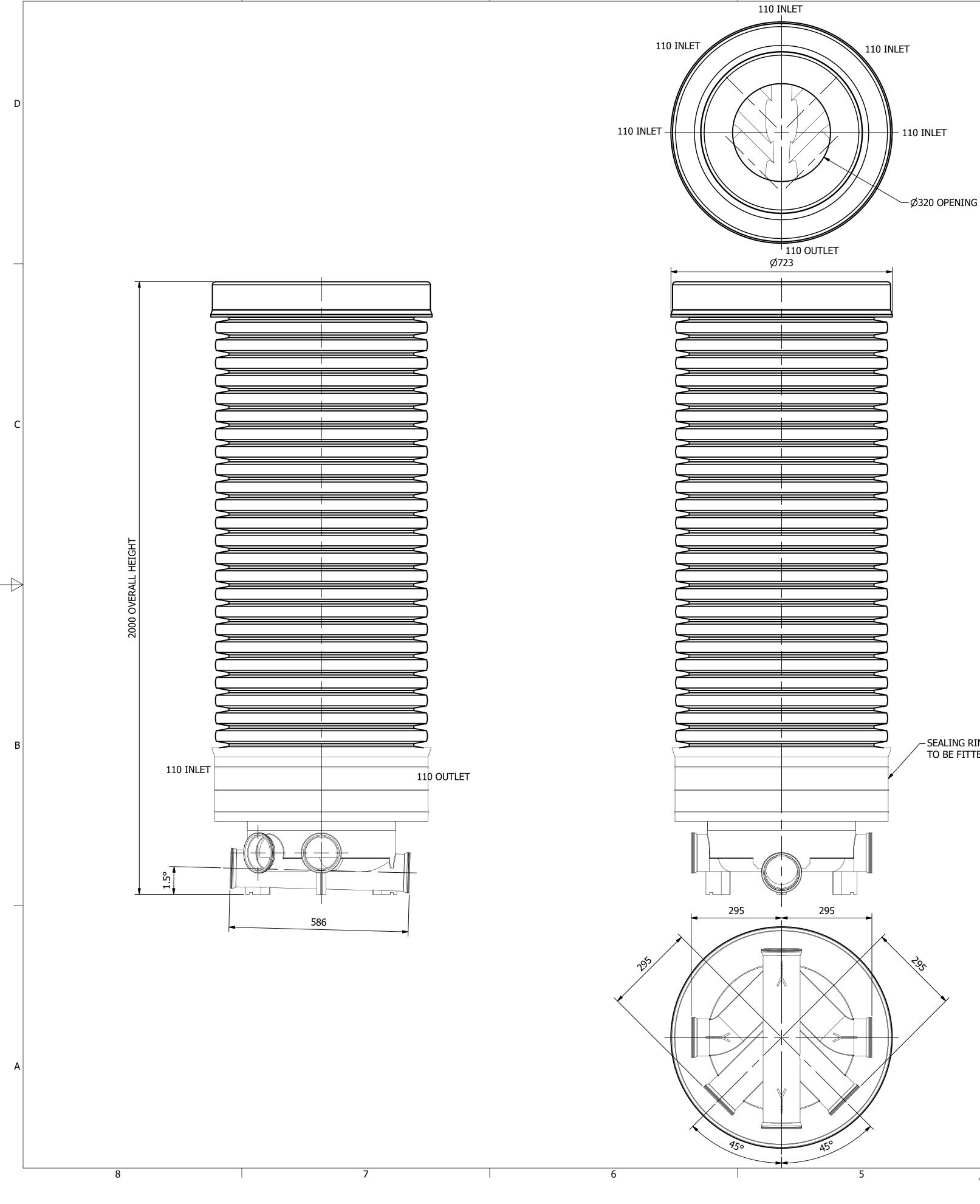
— SEALING RING (NOT SHOWN) TO BE FITTED ABOVE THE SECOND RIB
