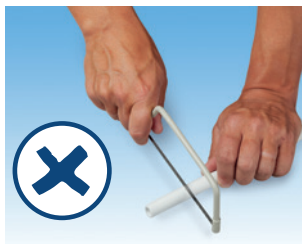
Figure 7: Don't use a hacksaw to cut Hep 2 O pipe
